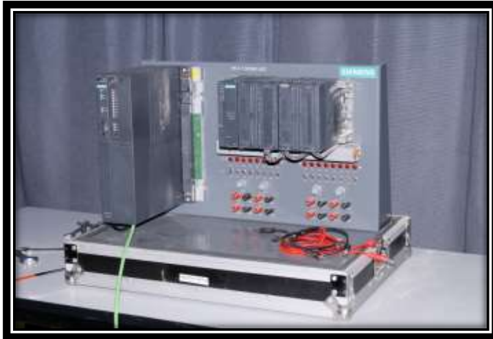
SIMATIC PCS-7 CONTROLLER (S7-400 PLC BASED HARDWARE)
